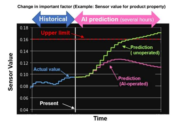
The AI system had predicted that the sensor value would exceed the upper limit if unoperated (green); the system automatically operated the control element to keep the value within the prescribed range (pink).
