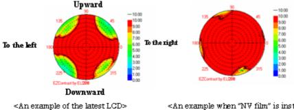
Although contrast is good no matter how far it is tilted in directions to the top, bottom, left and right, there are problems remaining when tilted diagonally. <An example when "NV film" is installed> Contrast is good, no matter in which direction it is tilted.
